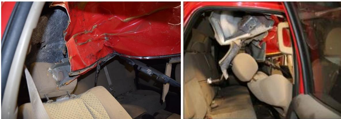
31. Below is an illustration showing the deformation of the roof windshield header. The maximum intrusion was 44” and the intrusion in the vicinity of Daniel Todd Arnold's head was 41”:
